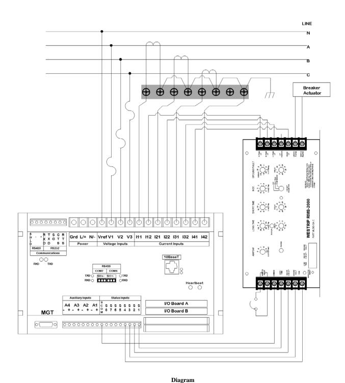
The above diagram shows the **WESTRIP RMS-2000** interfaced with the Power Measurements 7700 ION.
