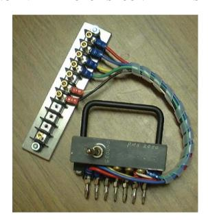
The Amptector Adapter Plug, shown above, is available from WESTRIP to facilitate the testing of the RMS-2000 on the Amptector Test Set.
