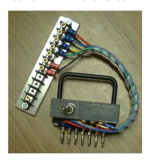
The Amptector Adapter Plug, shown above, is available from WESTRIP to facilitate the testing of the RMS-2007AF on the Amptector Test Set.
